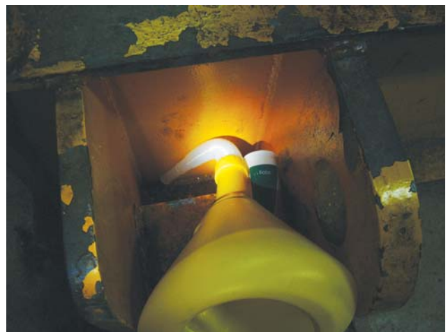
How not to store the funnel next to the pump! The funnel's spout is sitting in dirt and this will transfer along with the oil the next time the funnel is used.
