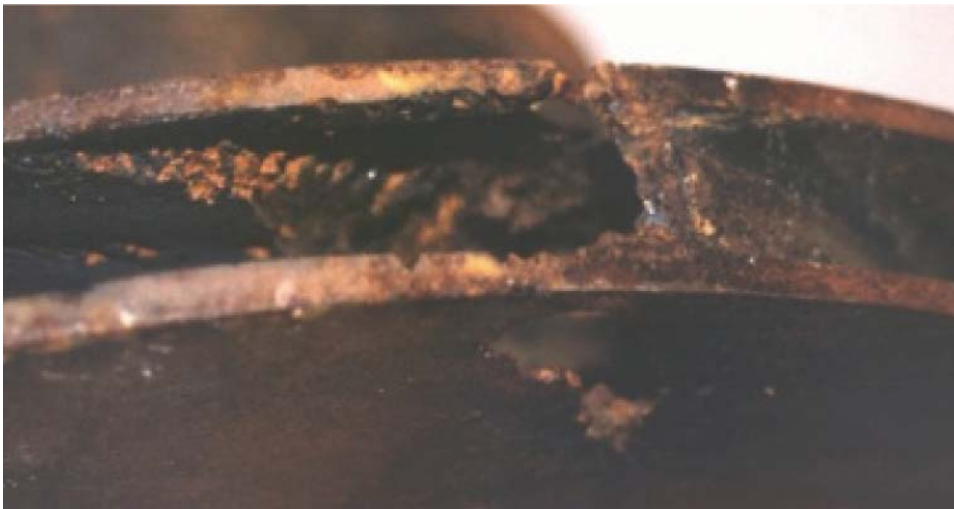
Figure #1: Courtesy of www.irrigationcraft.com/diagnosing_cavitation.htm . An example of extreme discharge recirculation damage.
