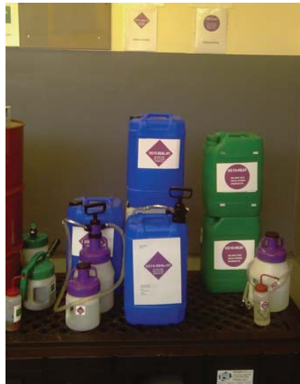
How the set-up should be for dispensing oil from drums into sealable containers, with colour-coding used to indicate products in the storage area.
