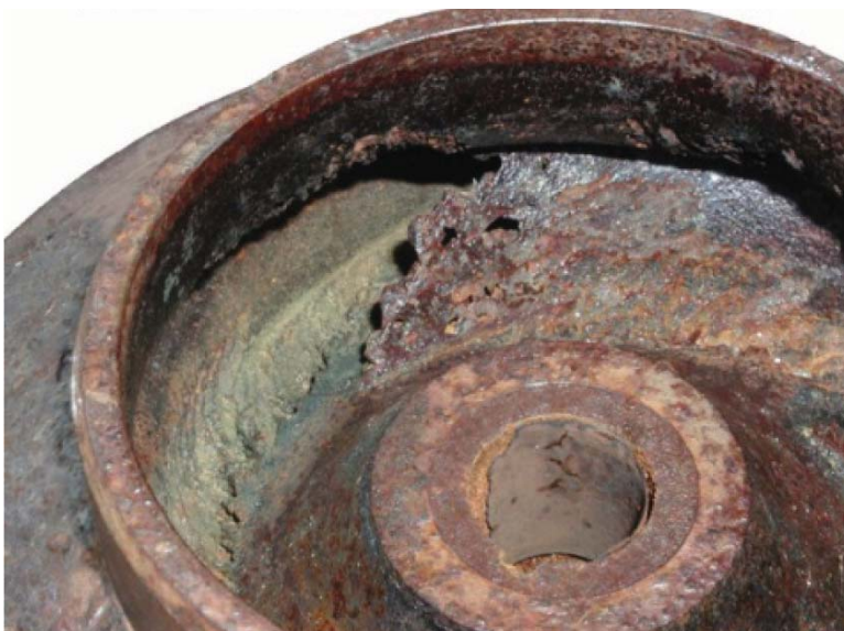
Figure #2: Courtesy of www.irrigationcraft.com/images/impeller_suction_cavitation_1b.jpg . This photo shows how suction cavitation has damaged the vane.
